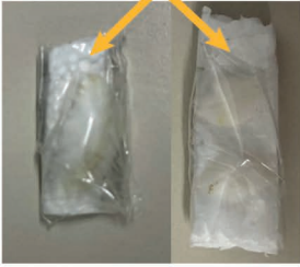
Figure 5. Preparation of otoliths for image acquisition using an X-ray microtomograph.
