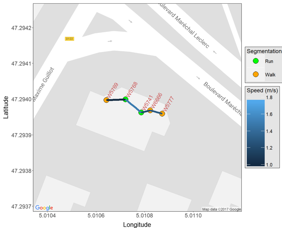
Fig. 12 Segmenting a worker trajectory in the run and walk segments to achieve semantic lines (the speed of a user is calculated in meter per second (m/s)). Value of speed is calculated between succeeding semantic locations. Based on the calculated speed values, the segments having the walk speed \leq 1.4 m/s are shown as “walk segments” in “orange” color. Whereas, the segments having the walk speed > 1.4 m/s are shown as “run segments” in “green” color
